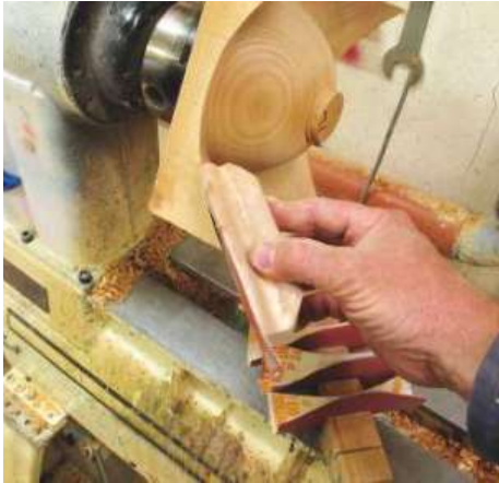
▲ Pic.19 Sanding the bottom of the piece is not easy as you have to consider the safest and most effective place to sand. I found that the majority of this had to be done with the lathe switched off
